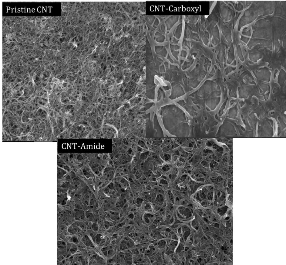
**Fig.4: Morphology of pristine CNT, CNT-carboxyl and CNT-Amide on IDT**
