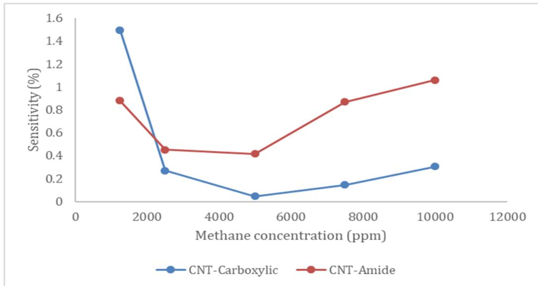
**Fig. 6: Sensitivity of CNT-Carboxyl and CNT-Amide network**
