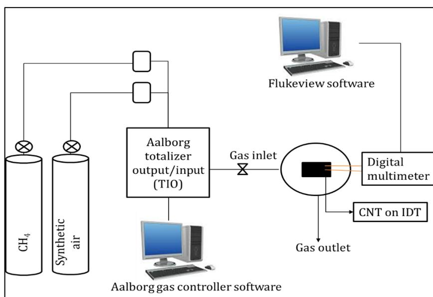
Fig. 2: Gas sensor set-up for detection of  $\text{CH}_4$  gas
