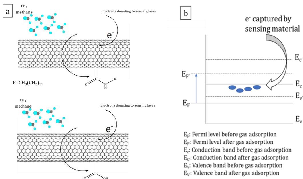
**Fig. 6: (a) Schematic mechanism on adsorption of  $\text{CH}_4$  gas on CNT sensing layer (b) band diagram of interaction between gas analytes and sensing layer (solid lines before gas adsorption, dashed lines after gas adsorption)**
