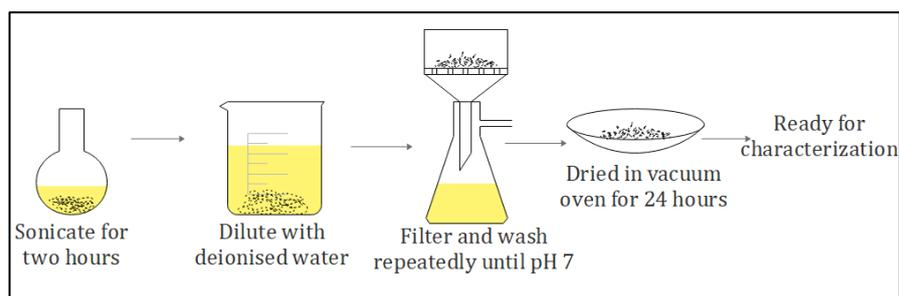
**Fig. 1: Preparation of CNT-carboxyl**
