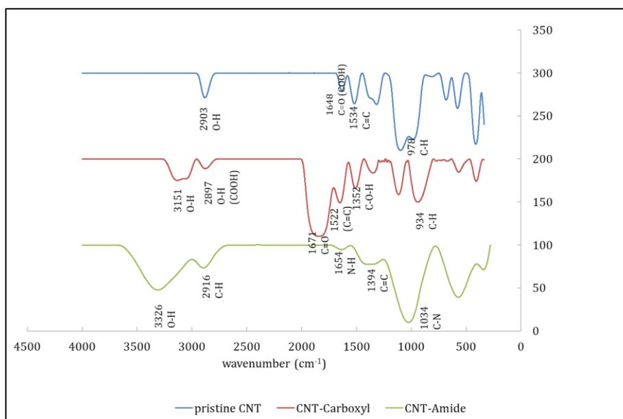
**Fig. 3: FT-IR spectra of pristine CNT, CNT-carboxyl and CNT-Amide**
