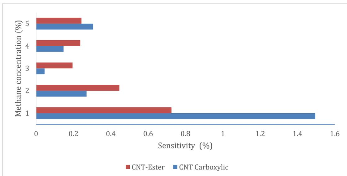
**Fig. 6: Sensitivity of CNT sample at different concentration of CH<sub>4</sub> gas**
