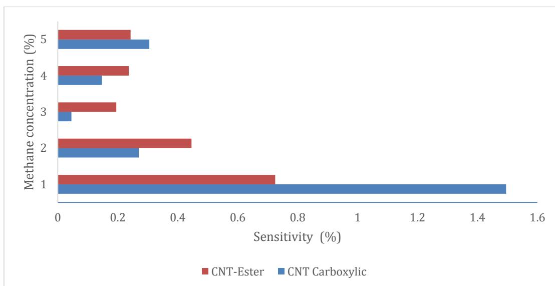
**Fig. 6: Sensitivity of CNT sample at different concentration of CH<sub>4</sub> gas**
