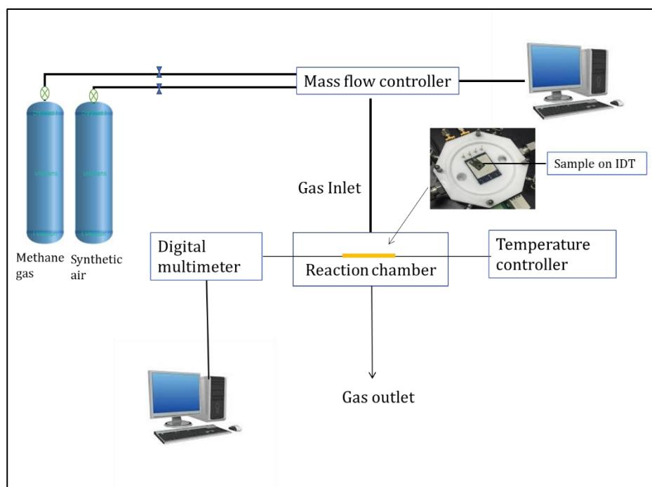
**Fig. 1: Schematic diagram of measurement set up**
