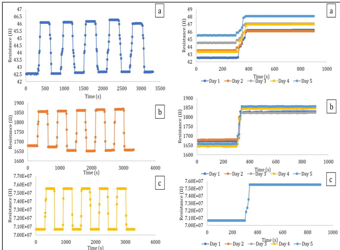
**Fig. 7: Repeatability and reusability of (a) pristine CNT (b) CNT-Carboxyl (c) CNT-Ester**
