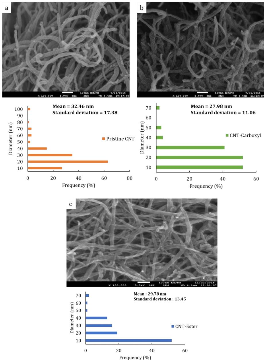
**Fig. 2: FESEM image (a) pristine CNT, (b) CNT-Carboxyl and (c) CNT-Ester**
