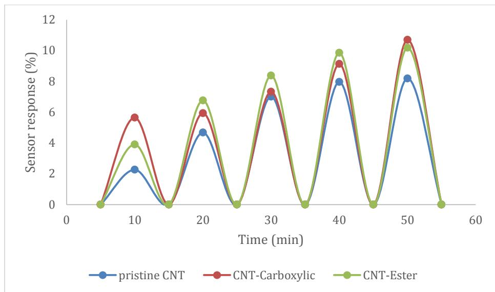
**Fig. 5: Response of CNT sample towards detection of CH<sub>4</sub> gas at different concentration**
