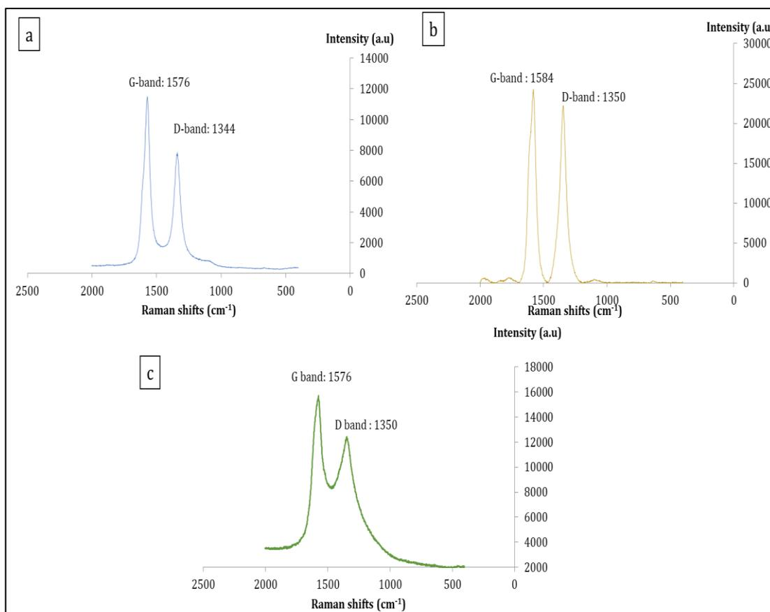
**Fig. 3: Raman spectra of (a) pristine CNT, (b) CNT-Carboxyl and (c) CNT-Ester**
