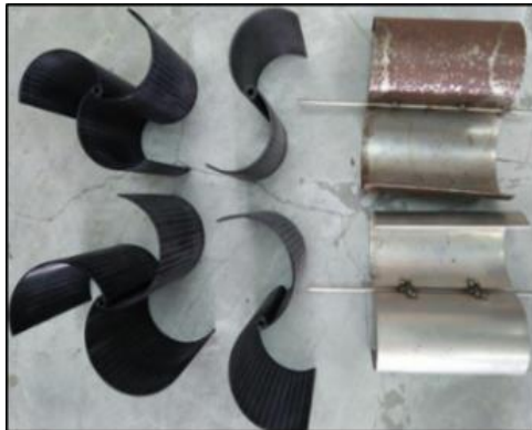
Fig. 4: Six models of Savonius wind turbine blade design and assemble design
